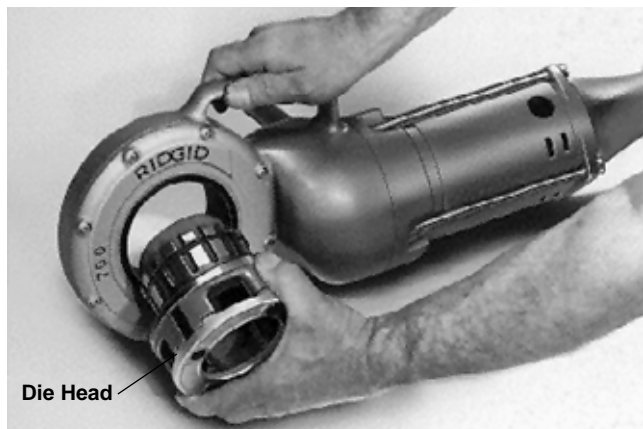
Figure 3 – Installing No. 12-R Drop Head Die Head
